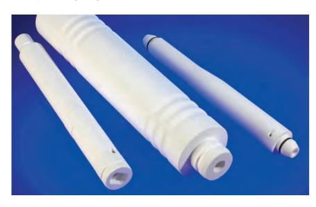
Larger hydrocyclone liners can be custom built in multiple sections using specially formulated joint technology. Proven for lengths up to 1.2m and internal diameters up to 250mm, the technology is scalable to larger sizes where requested.
